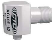
Ac146 Small Side Exit Sensor with built-in integral stud, 100mV/g, +/- 10% sensitivity.
